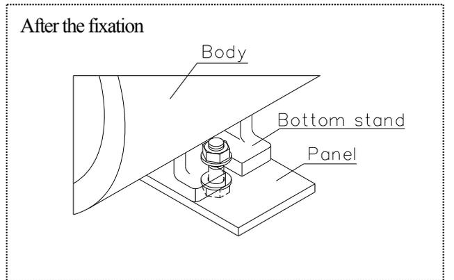
**○ Installation Procedure of the Locking Device**
