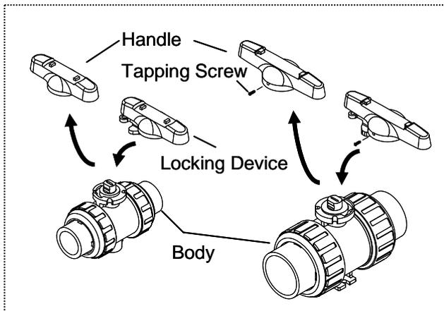
The location hole for the lock is already installed in the handle. (Table 1)
