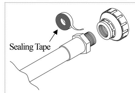
Socket End (End connector materials: PVC, C-PVC)
